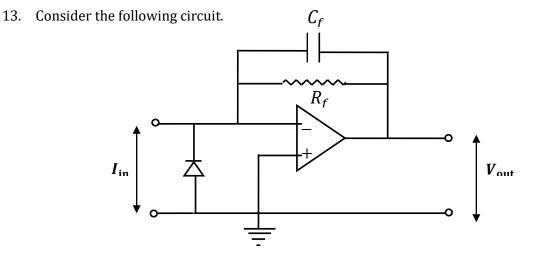
It is given that  $C_f = 100 \text{ pF}$ , and for  $I_{\text{in}} = 50 \text{ nA}$  D.C.,  $V_{\text{out}} = 1 \text{ V}$  D.C. Therefore, the bandwidth of the above circuit is
