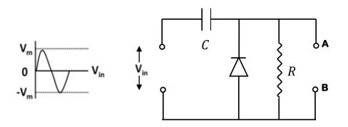
If the signal has time period  $\tau_S$  and the circuit has a natural frequency  $\tau_{RC}$ , then, in the case when  $\tau_S \ll \tau_{RC}$ , the steady-state output will resemble
