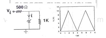
For  $V_i > 5V$ , the Zener regulates the output voltage by channeling the excess current through it self. Which of the following waveforms shows the current 'i' passing through the Zener diode?
