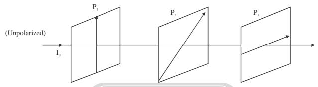
The pass axis of P<sub>1</sub> and P<sub>3</sub> are at right angles to each other while the pass axis of P<sub>2</sub> makes an angle  $\theta$  with that of  $P_1$ . A beam of unpolarized light of intensity  $I_0$  is incident on  $P_1$  as shown. The intensity of light emerging from P<sub>3</sub> is
